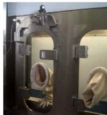
cRAB installed with Minncare Dry Fog nozzle
